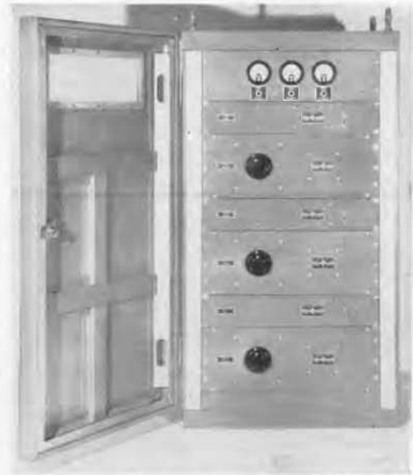
Figure 6. View of a three-phase, 18 KVA assembly of General Radio militarized regulators as used by Raytheon Manufacturing Company to provide constant line voltage for radar stations.
